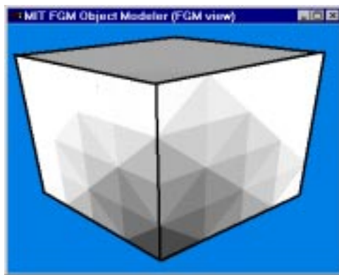
Figure 5. Cube consisting of 320 piece-wise constant FGM tetrahedra.
